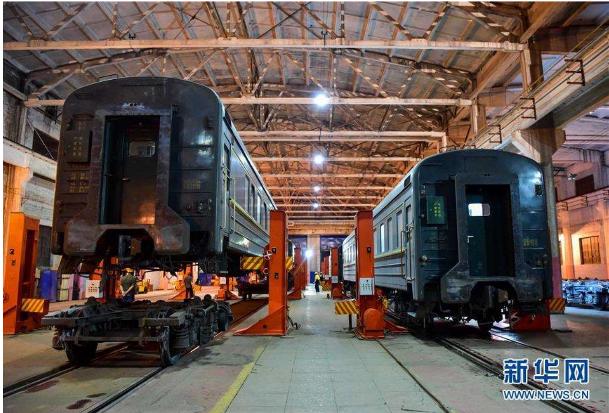
Changing train wheels at the Erenhot Port in Inner Mongolia in 2020. Image credit: Xinhua
